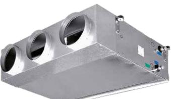
**Coil:** it is manufactured from drawn copper tube and the aluminium fins are mechanically bonded onto the tube by an expansion process. The Maestro Sabiana range is available with the combination of either 3 or 4 row coils (sizes  $1\div5$ ) with the possibility to add a 1 or 2 row coil (3+1, 4+1, 3+2, 4+2 versions for 4 pipe systems), and 4 or 6 row coils (sizes 6-7) with the possibility to add a 2 row coil (4+2, 6+2 versions for 4 pipe systems).
