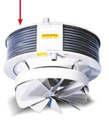
This is the most commonly used model; made of eight separately adjustable large louvres, shaped so as to be able to cover the whole outlet area and therefore adaptable for minimum to maximum heights. This diffuser allows the air to be directed more easily to the areas where it is required most, or conversely, if you do not require air to one particular corner you can close down one, two or three vanes and restrict the distribution.
